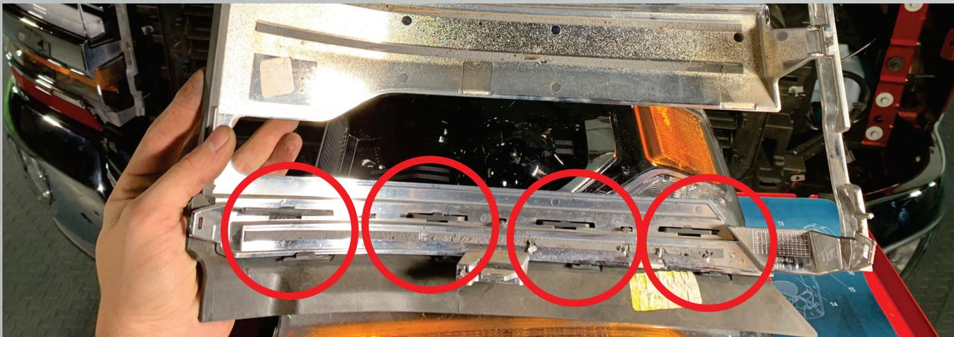
13. With the provided alcohol wipes, clean the indicated areas of the back of the trims and corresponding locations on the headlight assemblies.
