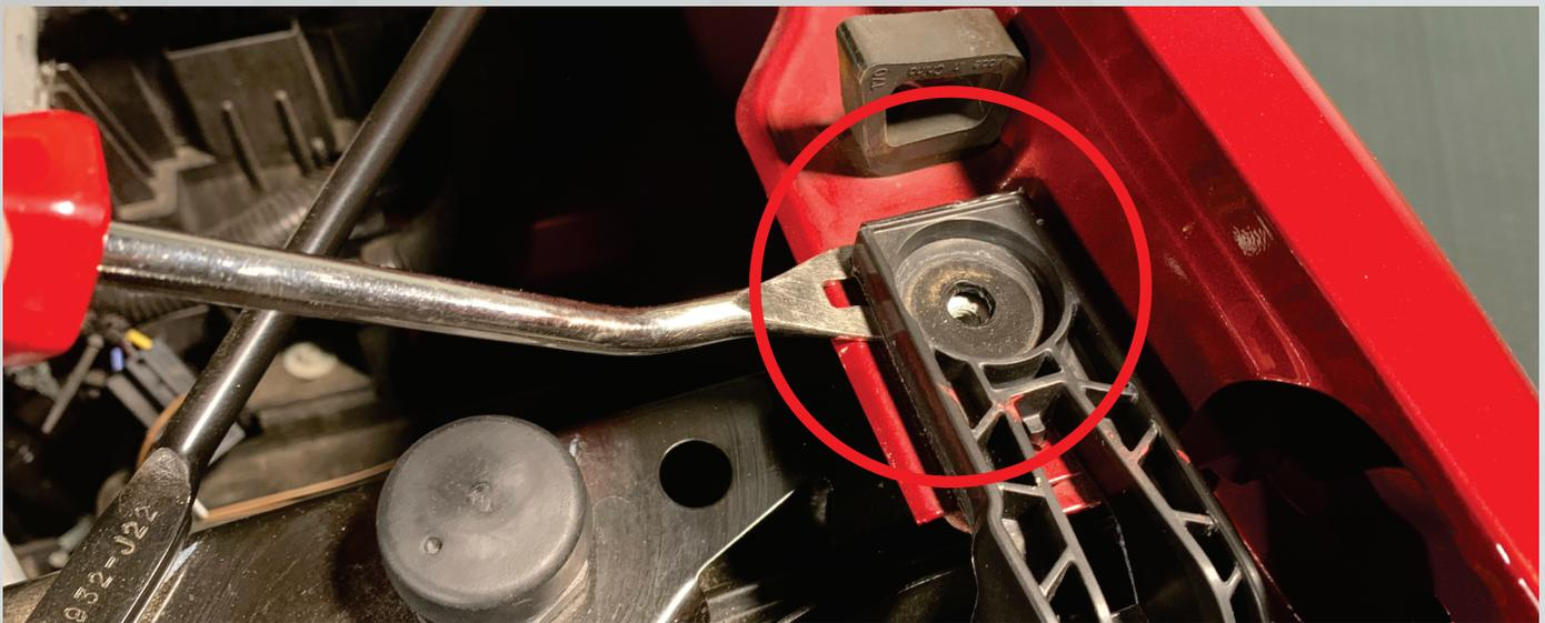
9. Unplug each headlight by pulling back on the red locking tab, then slide the connector off of the headlight.
