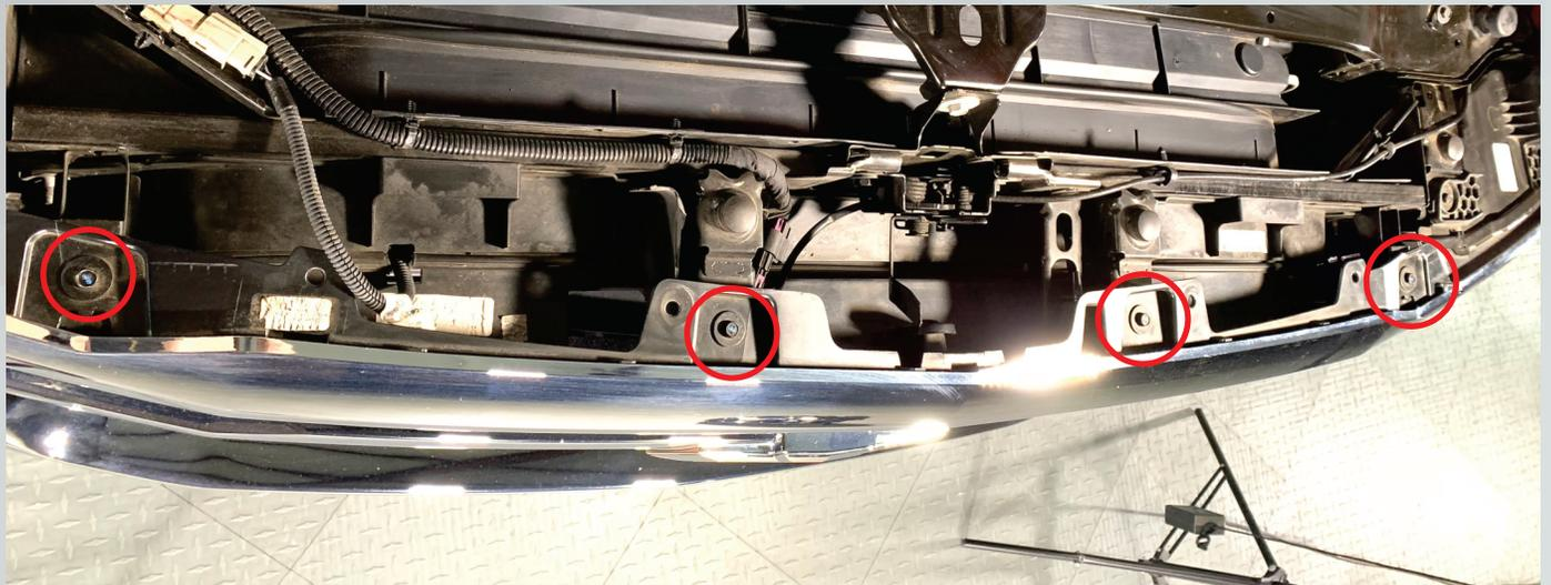
3. Using a trim tool or flathead screwdriver, pop the grille up and off of the tabs where the bolts were previously installed.
