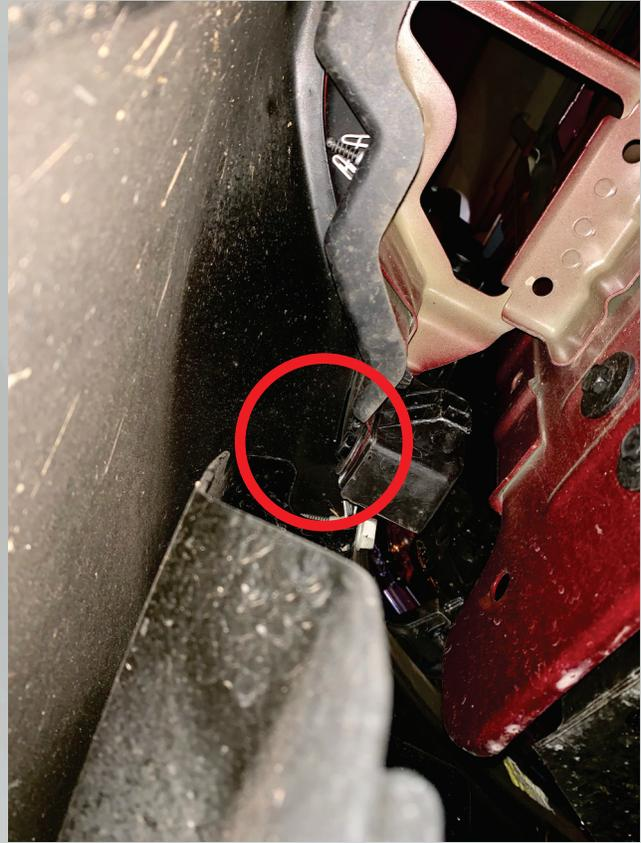
8. Back on top, use a trim tool or flathead screwdriver to pop the headlight bracket up and off of the slot in the fender retaining it.
