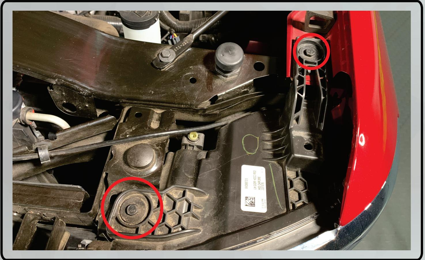
6. Remove the 10mm bolt from the bottom of the headlight behind where the stock grille was.
