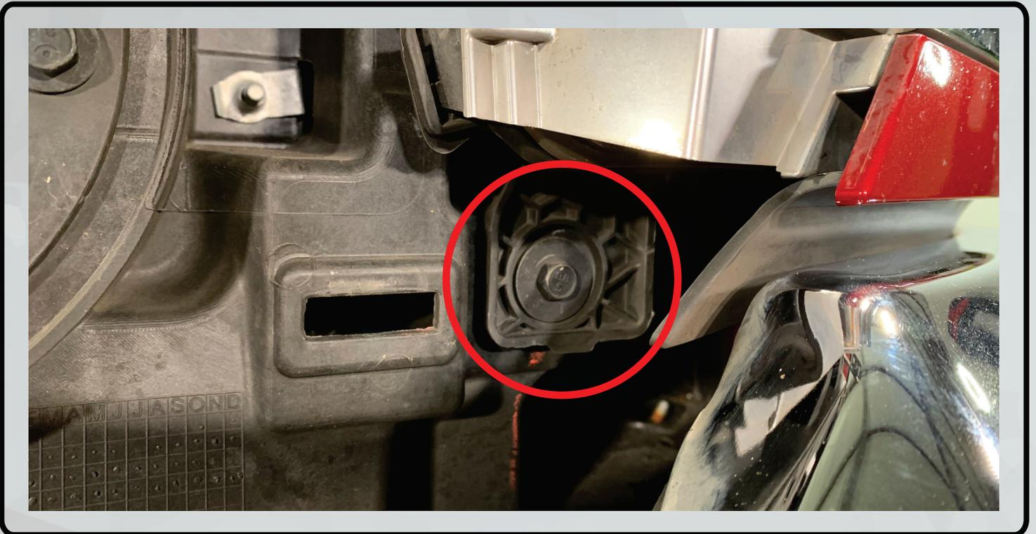
7. Using a T15 Torx screwdriver, remove the screw in the fender liner at the back of the bumper on each side. Reach up behind the fender liner to the side of the headlight and remove the 10mm bolt from each headlight.
