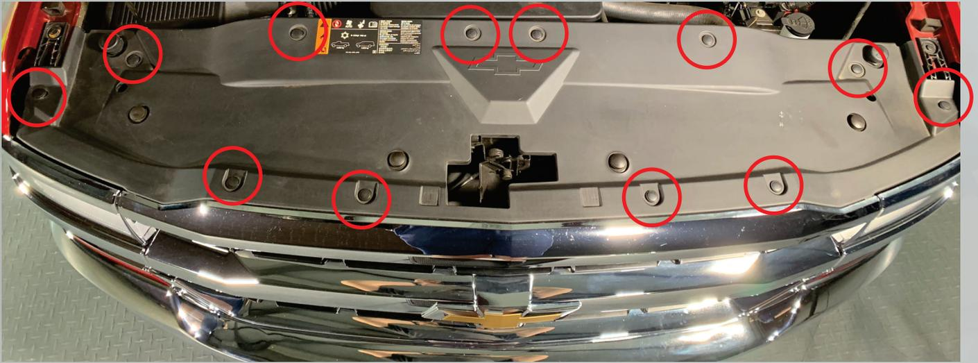
2. Remove the four (4) 10mm bolts holding the grille to the truck.
