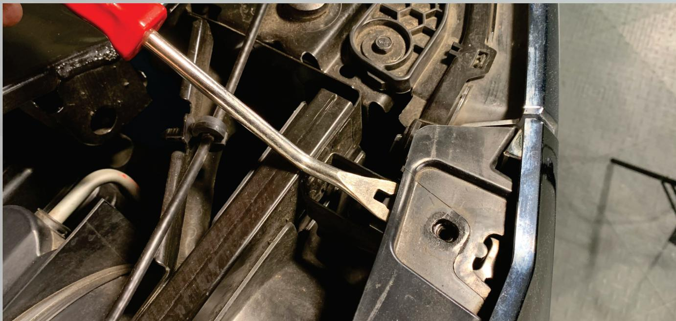
4. To remove the grille, firmly pull forward to release the push clips.
